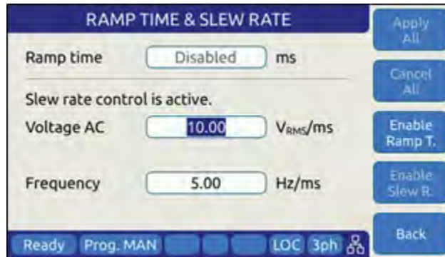
Figure 6-9: RAMP TIME & SLEW RATE SETTINGS Screen
