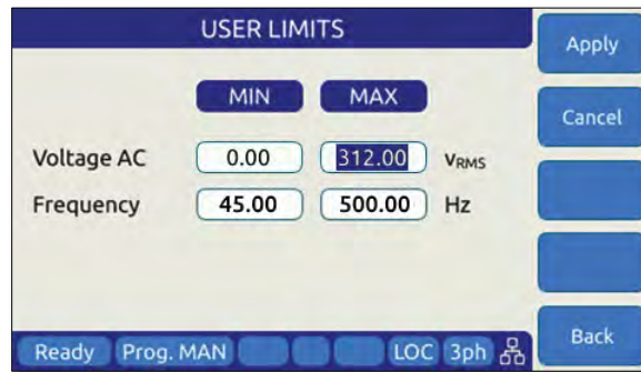
Figure 6-5: Enable Vac extended operating range to 312Vac
