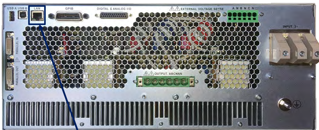
Figure 5-22: ADF Series® Rear Panel Layout
