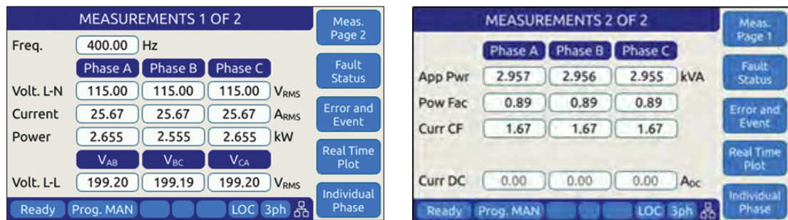
Figure 6-7: Three Phase Measurement Screens
