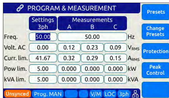
Figure 7-5: External Sync Input Sync Lost Status Indication
