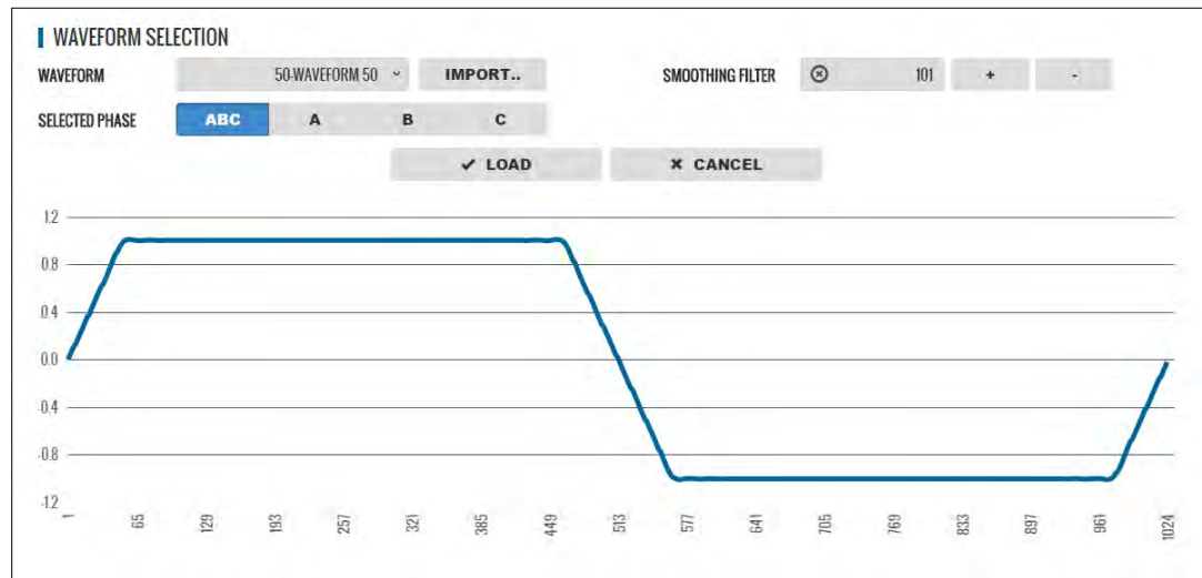
Figure 6-6: Same Waveform with maximum smoothing Filter Applied
