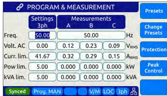
Figure 7-4: External Sync Input Sync Status Indication
